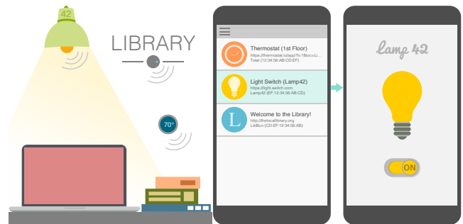
Figure 1: The Summon physical device browsing architecture. Peripheral devices like smart things (light bulb, thermostat) and beacons make their presence known by broadcasting information about themselves. The mobile phone Summon service scans the local vicinity, parses broadcast data, and displays to the user a selection of available user interfaces corresponding to the nearby devices. When a user selects an item from the list, the best possible interface for a given device is opened within the app, presenting a user interface that may interact directly with the device.
